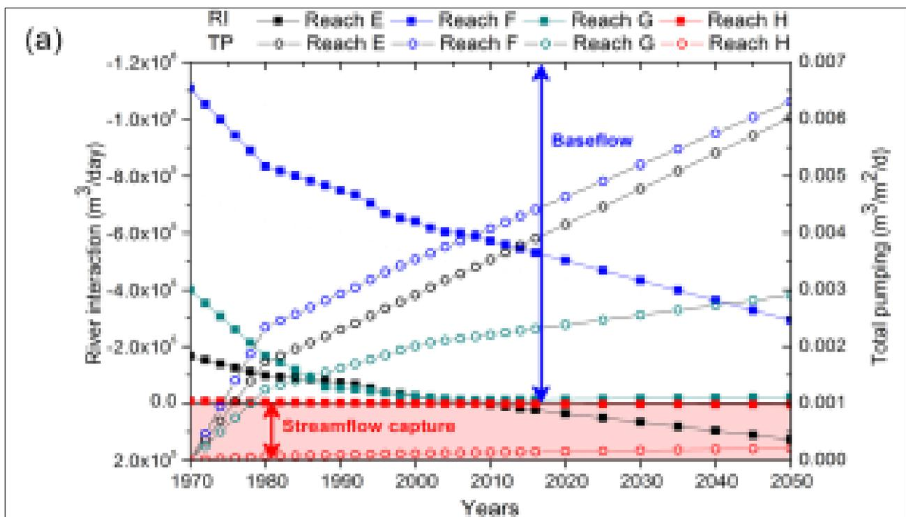
**Fig 1a:** Simulated response as generated simulating pre-monsoon river interaction (RI) as base flow or Stream flow capture using a hydro geologically-detailed regional groundwater flow model in the adjoining Gangetic alluvial aquifers for the Ganges River reach
