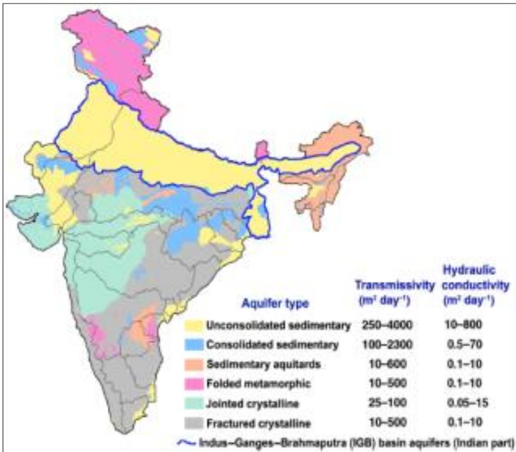
**Fig 4a:** Aquifer types, transmissivity ( $m^2 day^{-1}$ ) and horizontal hydraulic conductivity values ( $m day^{-1}$ )
