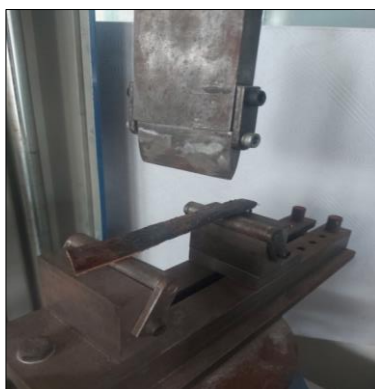
Plate 2: UTM machine loaded with sample for flexural test.
