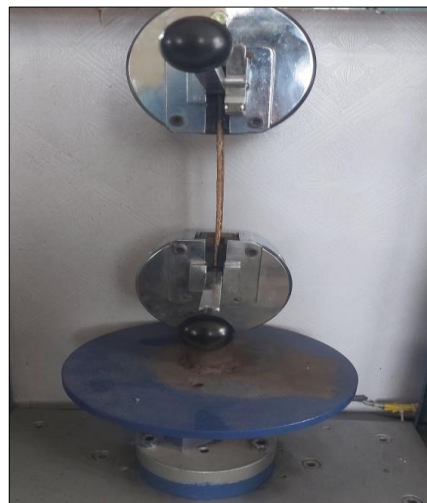
Plate 1: UTM machine loaded with sample for tensile test.
