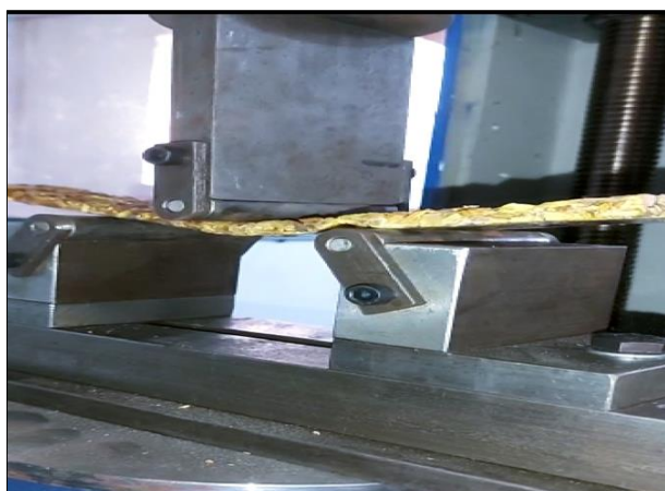
Fig 1: Sample placed between the load cells in the UTM for bending strength
