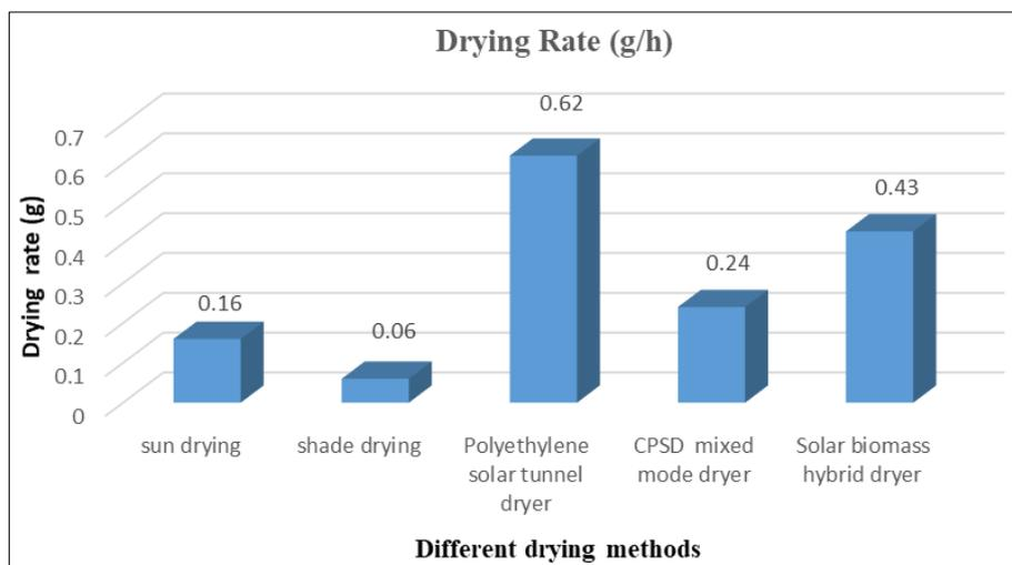
**Fig 4:** Drying rate of different drying methods
