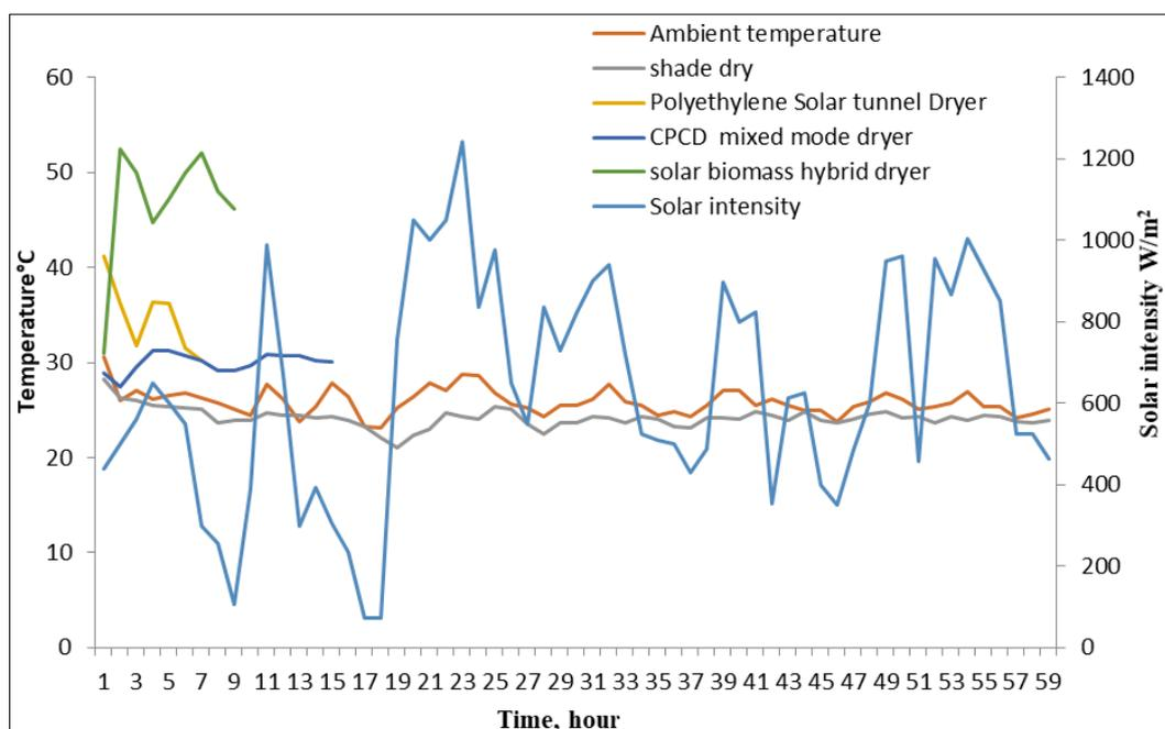
**Fig 1:** Solar intensity and drying temperature under different drying method
