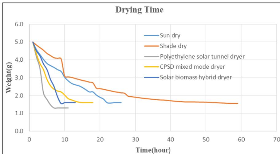
**Fig 3:** Weight reduction over a period of drying time
