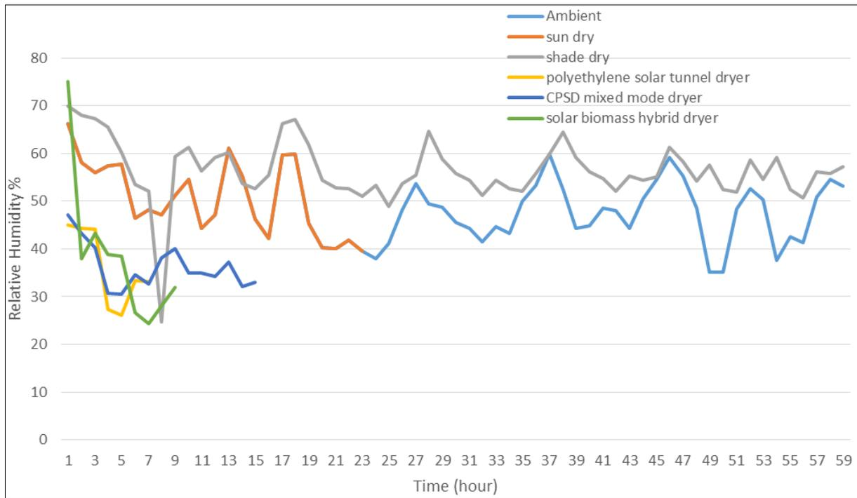
**Fig 2:** Experimental weather parameters under various drying methods (Relative Humidity %)
