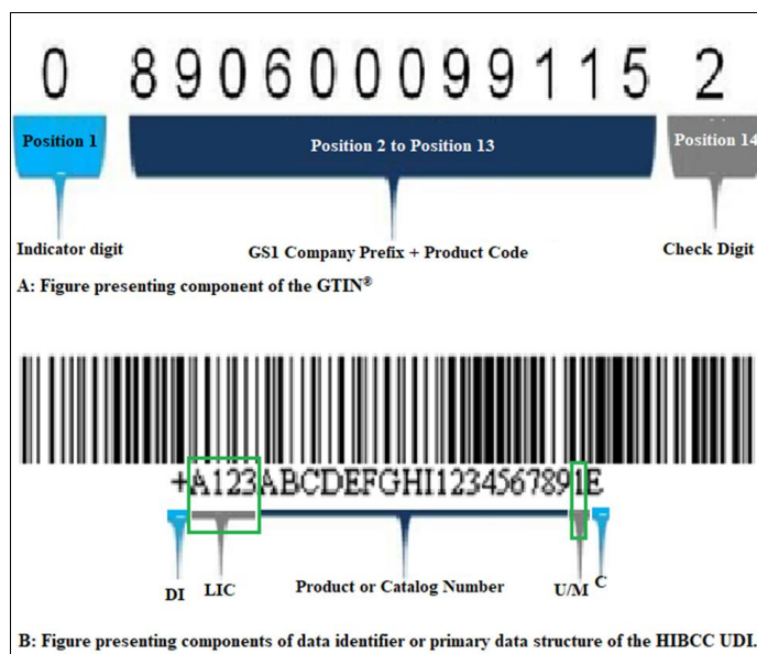
Fig 3: Figure presenting component of the GTIN® (A) and the HIBCC UDI (B).
