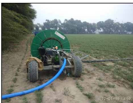
Fig 3, 4: Irrigation through Raingun at Central State Farm-NSC, Sardargarh, Rajasthan
