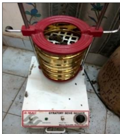
Fig 2: Sieve analysis of FYM
