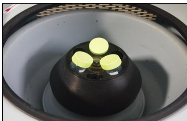
Fig (A): Centrifugation of filtrate for 5 min at 2500 rpm at room temperature
