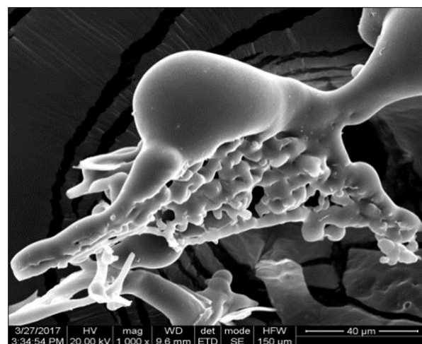
Fig 7: UTC sample examined at 1200Mag, HV-20.00KV, W.D-9.6mm and HFW-150μm showing smooth aggregates
