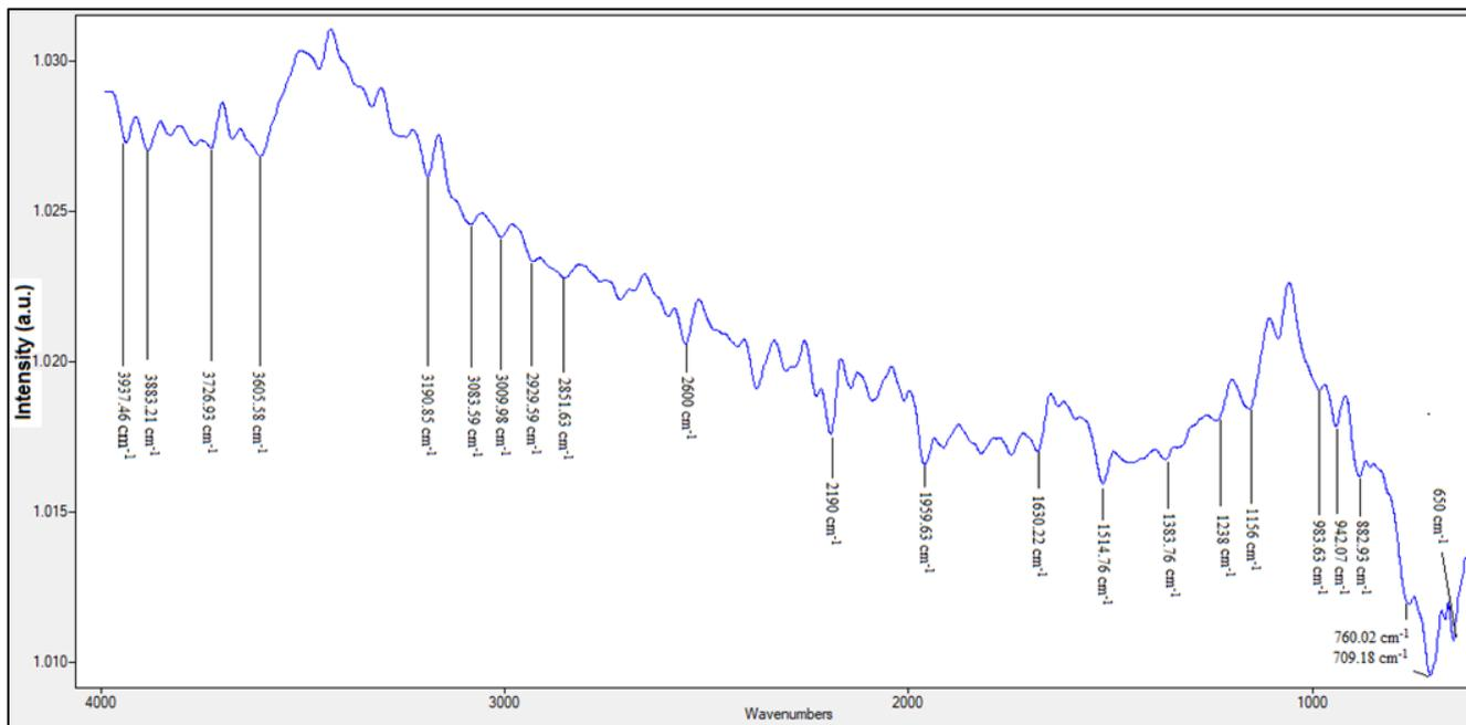
**Fig 4:** FTIR pattern of green synthesized nanoparticles by *Sonchus asper* (TiO<sub>2</sub> SA).
