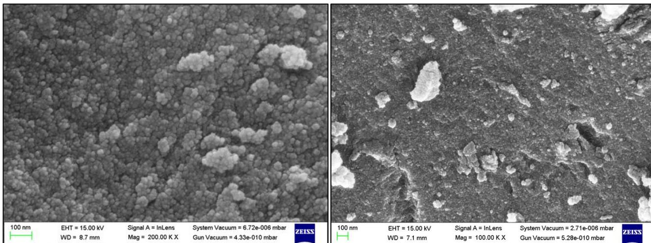
**Fig 2:** FESEM images of (A) chemically synthesized nanoparticles ( $\text{TiO}_2$ ) and (B) green synthesized nanoparticles by *Sonchus asper* ( $\text{TiO}_2/\text{SA}$ ).
