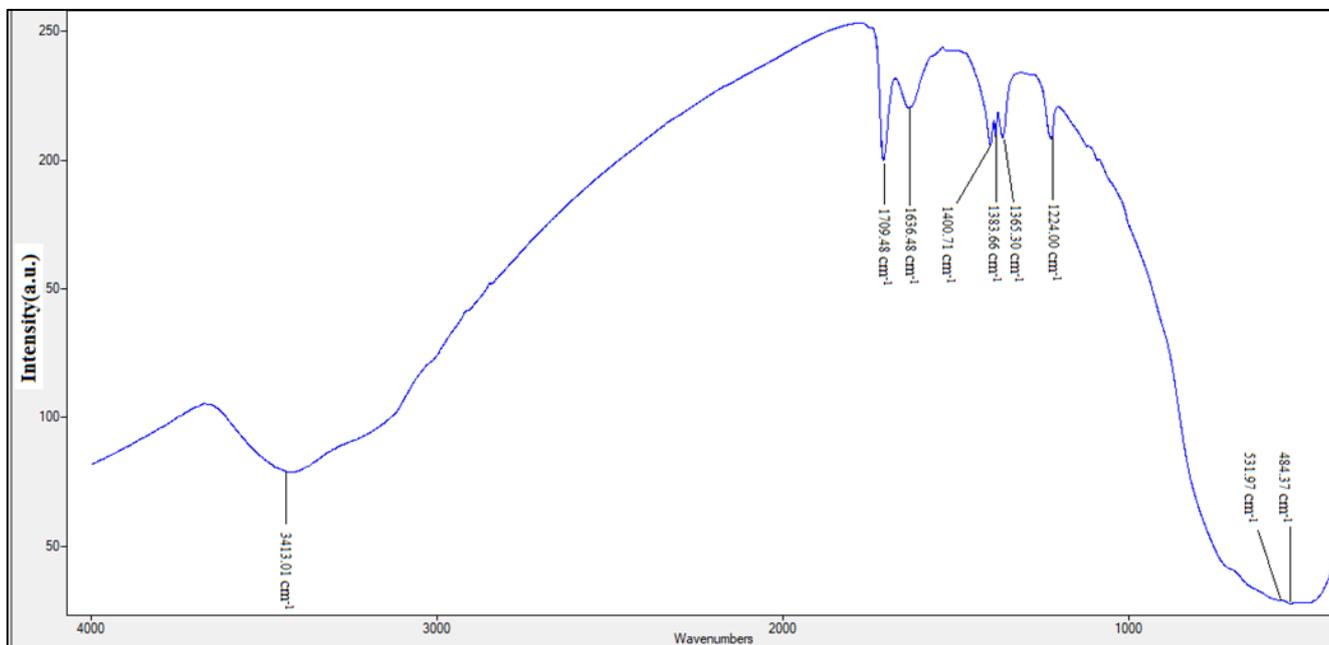
**Fig 3:** FTIR pattern of chemically synthesized  $\text{TiO}_2$  nanoparticles.
