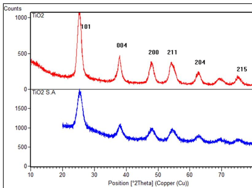
**Fig 1:** XRD pattern of chemically synthesized nanoparticles (TiO<sub>2</sub>) and green synthesized nanoparticles by *Sonchus asper* (TiO<sub>2</sub>).
