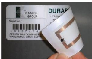
**Smart labels:** Smart labels differ from RFID tags in that they incorporate both RFID and barcode technologies. They're made up of adhesive label embedded with an RFID tag inlay, and they may also feature a barcode and/or other printed information.
