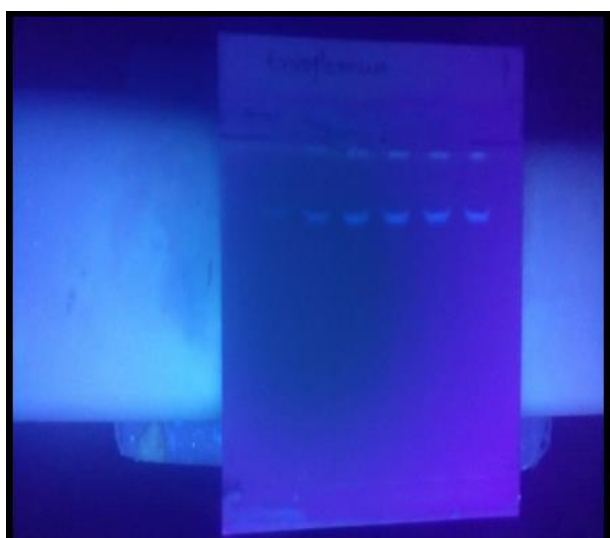
Fig 12: TLC plate showing linearity of enrofloxacin under UV
