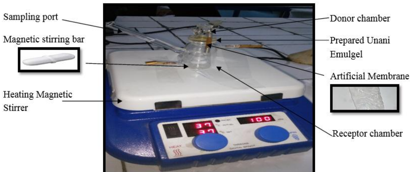
Fig 1: In vitro Release /Permeation Study of Emulgel by Franz Diffusion Cell Apparatus
