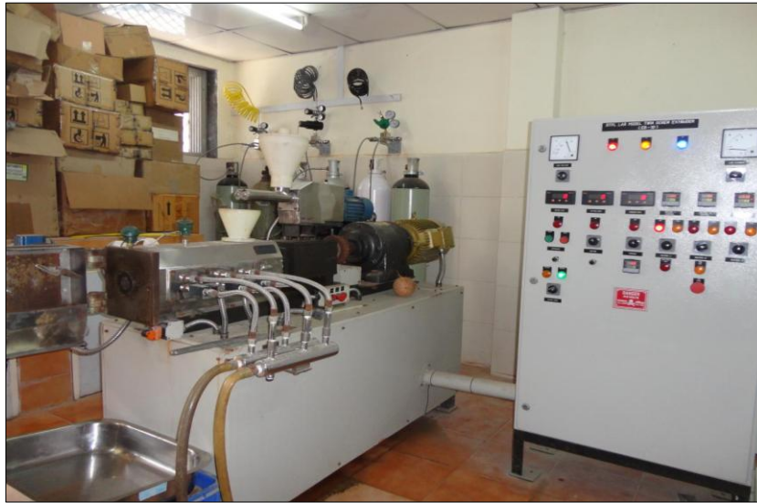
Fig 1: Twin screw extruder (Department of fish processing, Central Institute of Fisheries Education, Mumbai)
