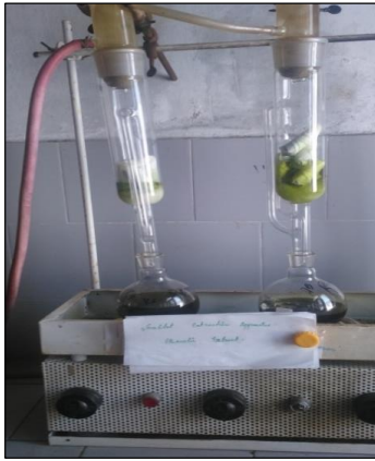
Fig 5: Soxhlet extraction apparatus
