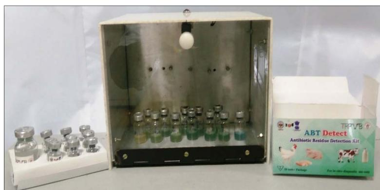
**Fig 1:** Schematic representation of the MIA named ABT Detect kit along with portable incubator
