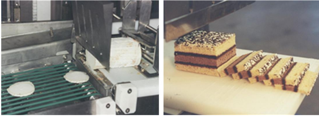
Fig: Difference in cutting slices of a bakery product cut with and without ultrasound
