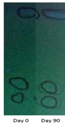
Fig 4: Fingerprints of n -hexanic extracts of the syrups at the date of manufacture and 3 months later by TLC; Eluent: n -Hexane – ethyl acetate - méthanol 7:2:1 Revelation under ultraviolet lamp at \lambda = 365 \text{ nm}
