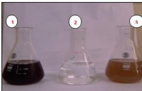
Fig 1: 1- Green seaweed water extract. 2- AgNO 3 3- Green Seaweed synthesized silver nanoparticles solution
