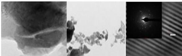
**Fig 9:** TEM, HRTEM, SAED of Yashad Bhasma prepared by incineration with electric muffle furnace heating
