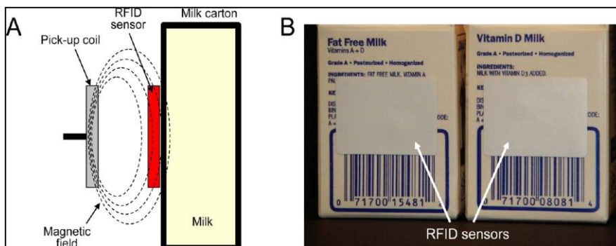
Fig 3: RFID sensor layout for demonstration of determination of milk freshness: (A) schematic of sensor positioning onto milk carton and sensor-response readout with a pick-up coil; (B) photograph of milk cartons with attached RFID sensors.
