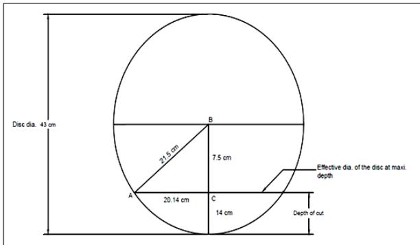
Fig 4: Determination of cutting width of disc by geometrical method
