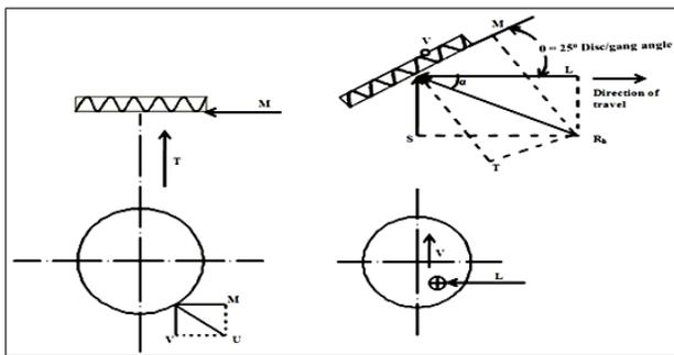
Fig 5: Force acting on wavy coulters disc
