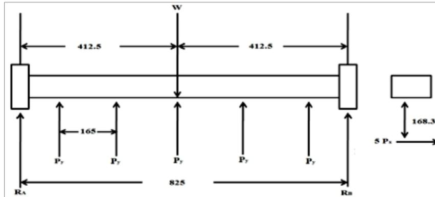
(a) Vertical forces Note: all dimensions are in mm, (b) Horizontal force
