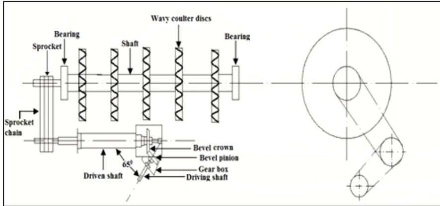
Fig 3: Power transmission system of vertical tillage implement
