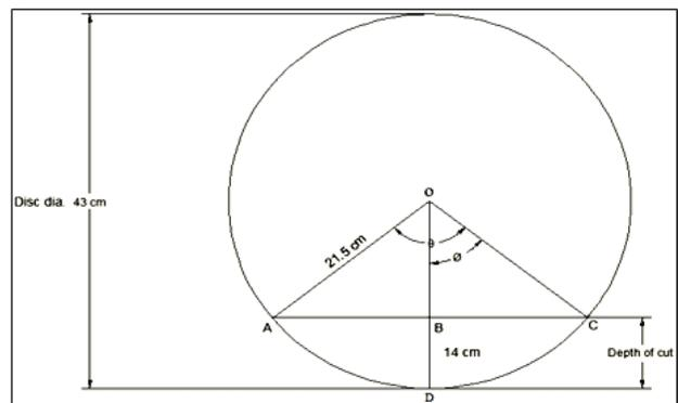
**Fig 1:** Schematic of surface area of disc under soil
