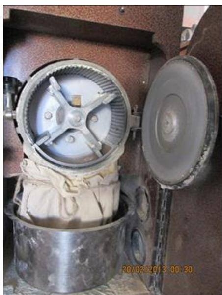
Fig 2: Hammer Mill
