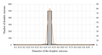
**Fig 5:** Histogram of the droplet size distribution at a ratio of emulsifiers Dimodan OT and Ceteareth 20 1:6.
