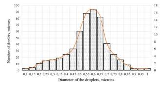
**Fig 2:** Histogram of the droplet size distribution at a ratio of emulsifiers Dimodan OT and Ceteareth 20 1:3.
