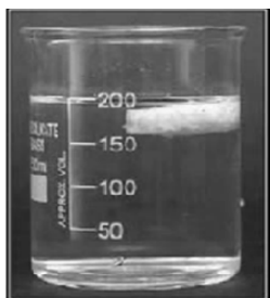
Fig 1: The formulation M6 containing drug and polymers remained buoyant for more than 12 h
